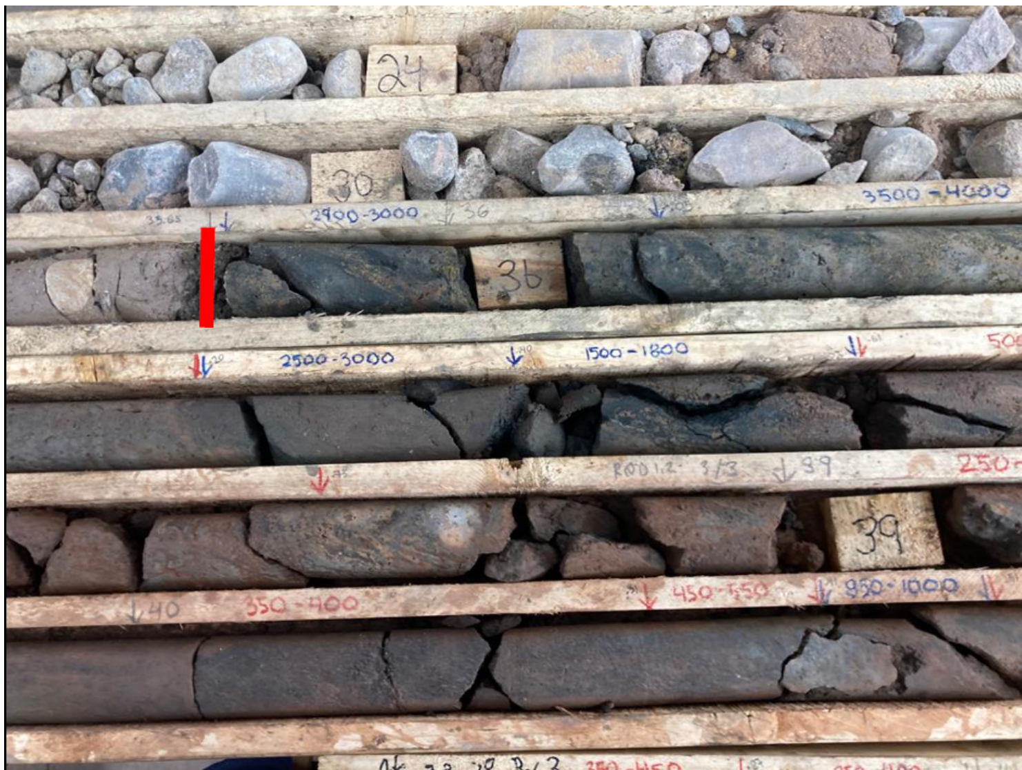
FIGURE 2 – Elevated radioactivity directly beneath overburden, drill hole AK22-038 (overburden/basement contact defined at red line)
