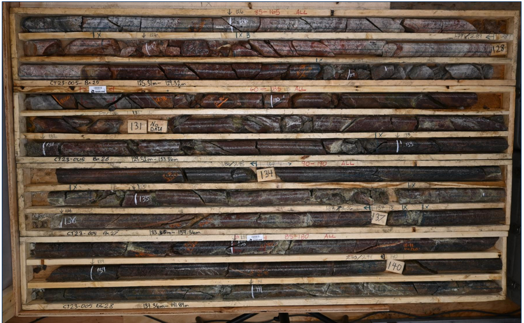
Figure 2: CT23-005 (125.3 - 141.8 m); overlapping quartz, hematite and clay alteration
