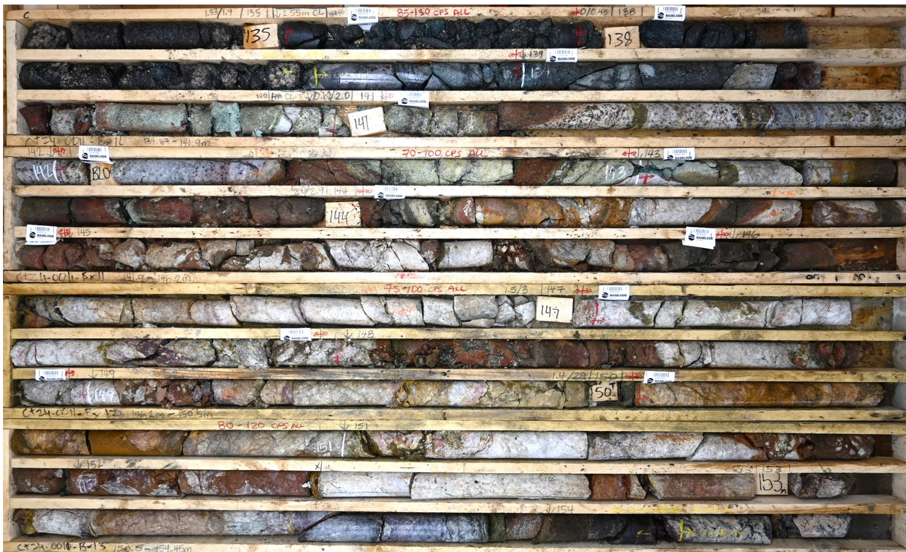
FIGURE 4 – CT24-011, 134.7 to 154.5 m, overview of part of structural system and hydrothermal alteration
